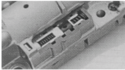
Fig. 18: Thermostatic control valve (cut-away)
