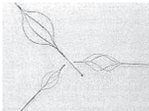
Figure 6: Examples of Nitinol baskets with distal ends shape set into the final configuration.
