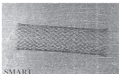
Figure 6: Fluoroscopic image of the Cordis Nitinol SMART stent, which was approved for biliary use in the US in late 1998. It is laser machined from tubing and expanded to final configuration. It is thermally deployed into the body by proper control of the A_f temperature. The fine features allows optimal flexibility and gentle chronic outward force.
