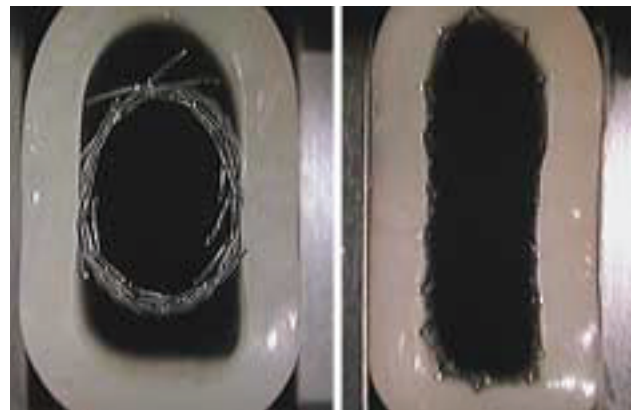
Figure 11. Two commercially available SE stents of the same nominal diameter are deployed into a flattened lumen. The stent on the right exhibits excellent wall apposition, while the one on the left does not.
