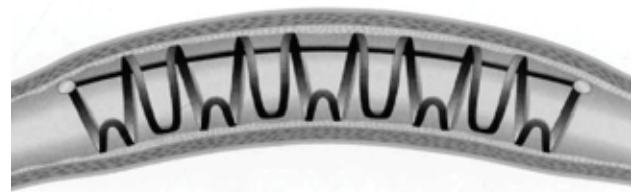
Figure 5. Cook GRII, formed from stainless steel sheet, featuring an axial backbone with integral gold markers.
